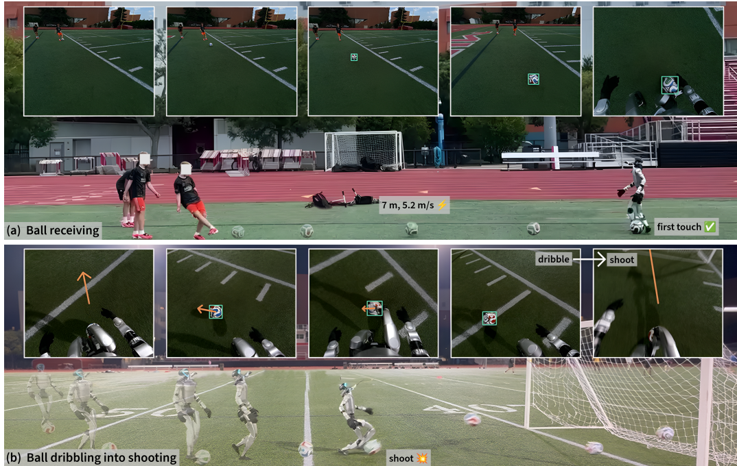
Fig. 1. Agile soccer skills with Joga , a full-stack system for humanoid dribbling, shooting, passing, and receiving. A custom 2-DoF actuated neck enables active vision. Our real2sim2real techniques on perception and dynamics help transfer fast, precise whole-body behaviors learned in simulation via reinforcement learning to the real world. In (a), the robot makes a “perfect” single first touch with the outside of the right foot to receive a fast incoming pass of 5.2 m/s. In (b), the robot dribbles from 10 m away and directly strikes the ball into the goal with a commanded ball speed of 10 m/s. Green boxes show detector outputs and orange arrows show ball joystick commands. Nolan: Need to show WB-UAN closes the sim-to-real gap. Current results only show it improves dribbling speed and ball control.
